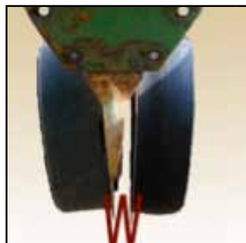
Figure 4. Worn disks affect furrow shape.
