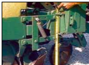
Figure 3. Down-pressure springs hold units in ground.
