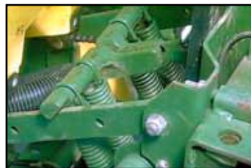
Figure 2. Set the bar at a ht. of 20" for level planter.
