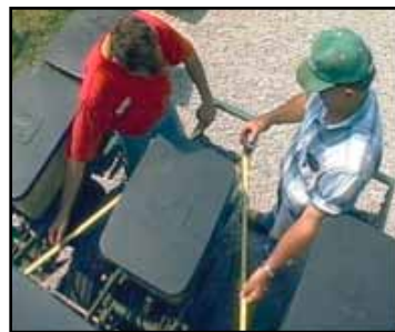
Figure 1. Checking for bent or twisted row unit.
