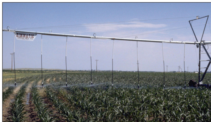
Figure 1. Precision nozzles increase irrigation efficiency under limited water supply. Photo courtesy of G.W. Buchleiter, www.Bugwood.org .
